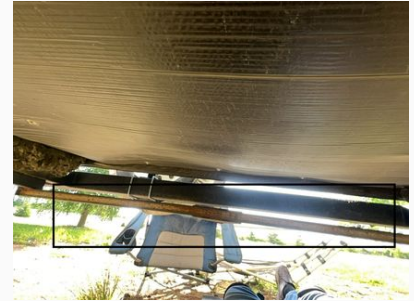
Towbar shows signs of rust.
