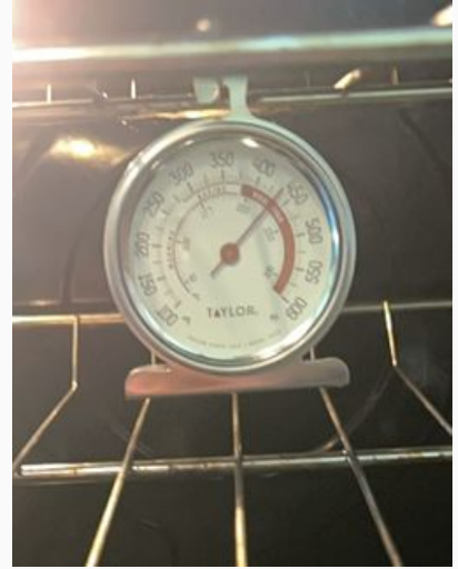
Oven Temperature set to 425F, result 425F
